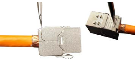
⑩.Press down the retainer for 360 degree shielding
