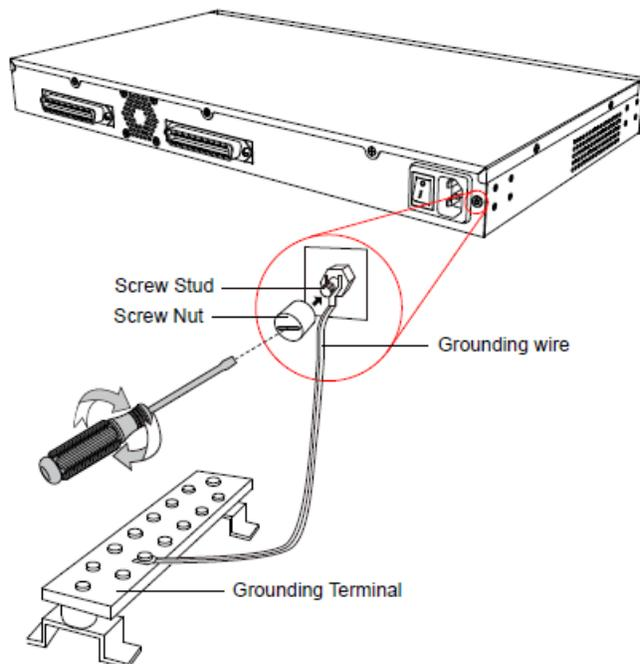
1. Tighten the provided M3\*5 screw stud into the grounding port on TA device.
