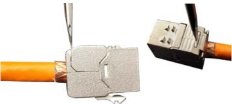
⑩.Press down the retainer for 360 degree shielding
