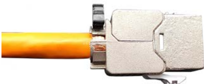
⑨.press both covers of the keystone jack to contact the cable
