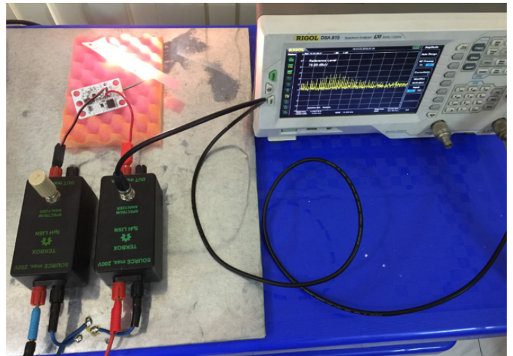
Picture 13 – Example: conducted emissions, pre-compliance measurement of an automotive LED driver using two LISNs
