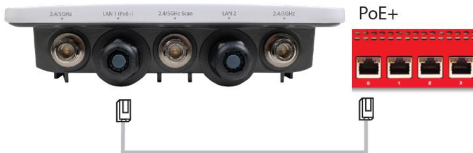
Access Point connected to switch with PoE+ power
