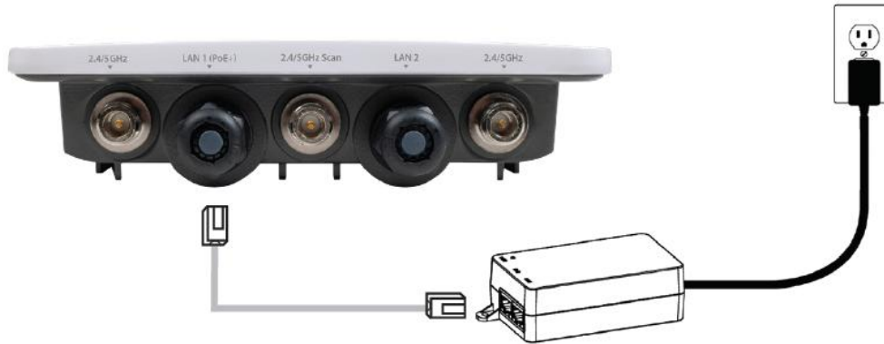
Access Point connected to PoE+ injector
