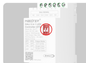
Select output mode via PIN switch
