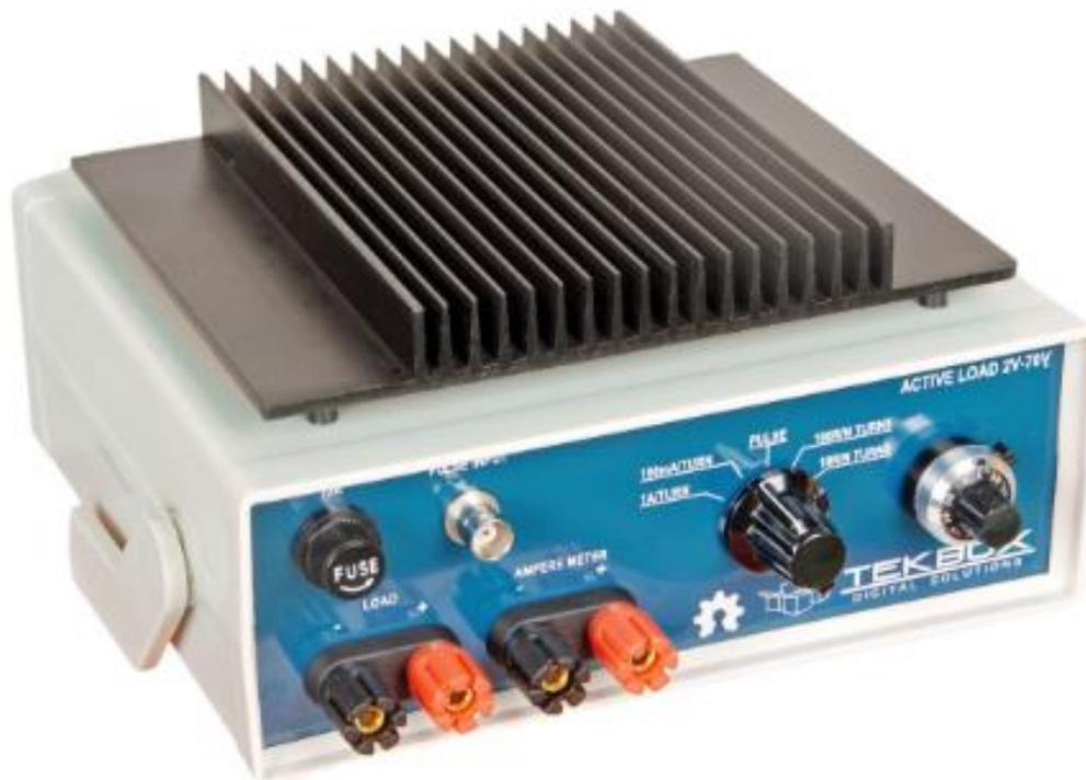
The TBSOH02 operates from 2V to 70V. The maximum current is up to 10A, however it has to be taken care that the maximum power without additional cooling is limited to 25W. A fan, attached to the heat sink, can increase the maximum power rating up to 100W.
