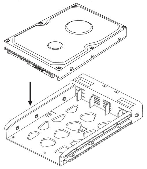
Step 2: Align the six steel balls on the bracket as shown in the illustration with the screw holes on the hard disk and insert the hard disk Insert the hard disk holder from top to bottom.
