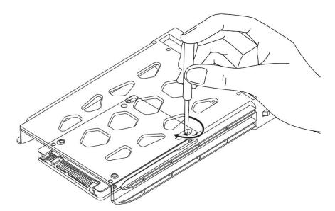
Step 3: Install and tighten the screws from the back as shown, and reinstall the bracket into the housing.
